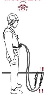
**WARNING!** For HORIZONTAL PROGRESSION a SPARROW TWIN lanyard must be used. **Always use both strings of the lanyard to pass an intermediate point!**
